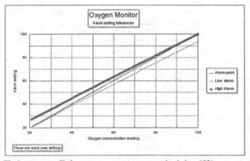
The instrument will alarm at any oxygen concentration below 18%
