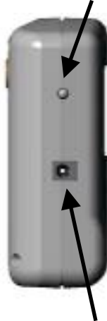
Infra Red (IR) output LED
