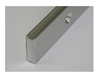
Note: the example above has a curved recess along the top, this is not necessary but the straight recess along the bottom is necessary.
