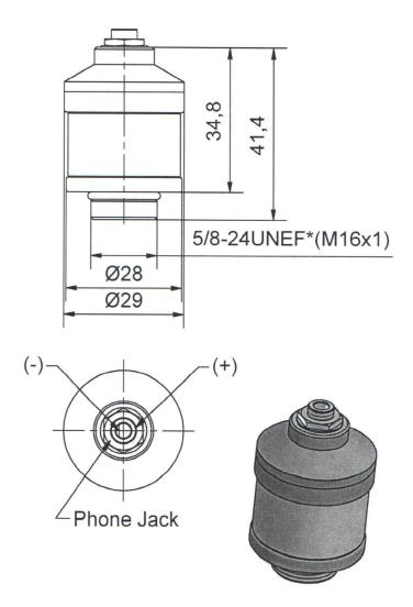
General tolerances ISO 2768-c Color of housing parts: RAL 7040
