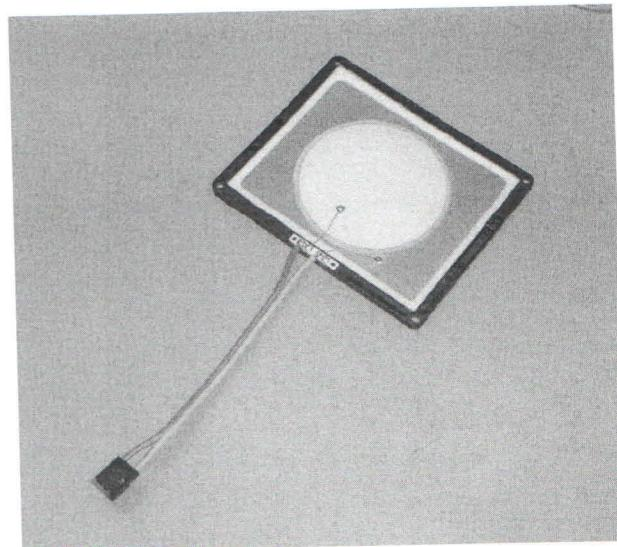
8. Mount the transducer to the transducer mounting board. Space the transducer away from the board using a nut.
