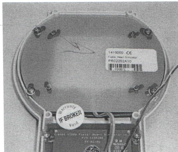
20. Affix a serial number label to the back of the transducer assembly.
