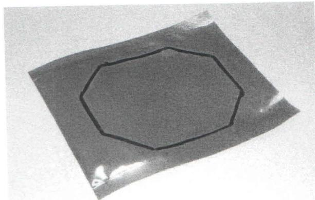
2. Seal the edges of the transducer cushion, leaving a small gap for filling.
