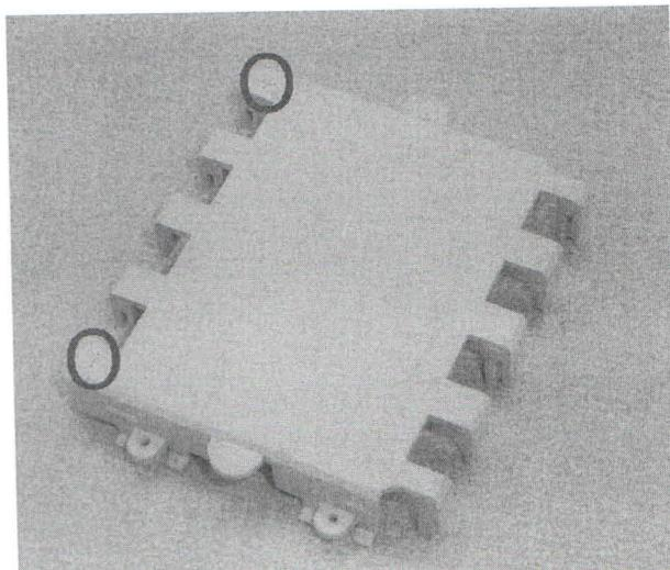
3. Using the retaining hooks, located at each end of the battery compartment, insert the compartment into the lower case.
