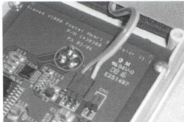
14. Cut a length of ribbon cable to 150mm. Affix a 2 pin M22 connector.
