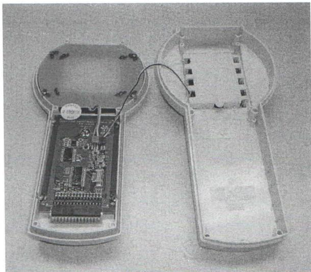
19. When the unit is working as expected, use Tamper Evident Seal on the exposed nuts and screw heads.
