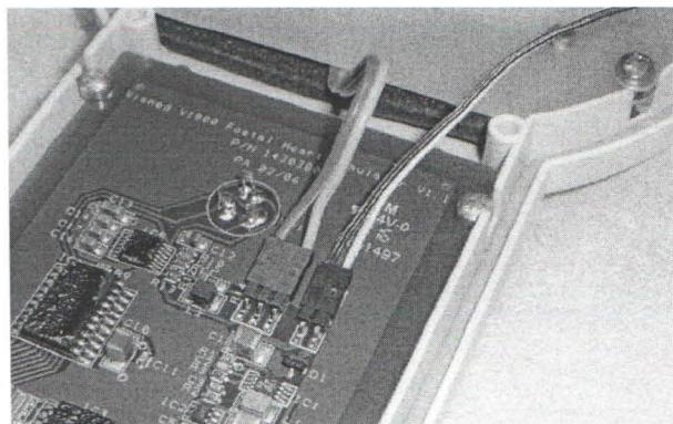
17. At this point, test the unit. Insert 4xAA batteries and fix the case halves together.
