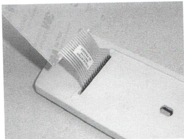
3. Remove the protective backing from the keypad to expose the adhesive backing.
