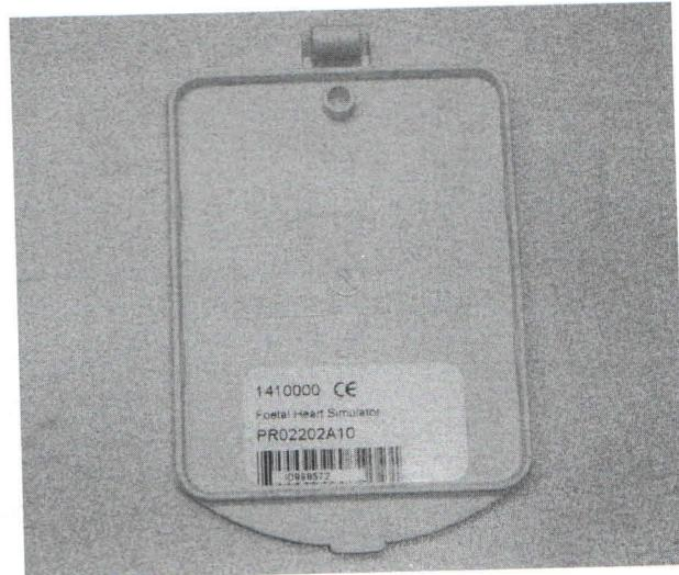
23. Affix a trimmed serial number label to the inside of the battery compartment.
