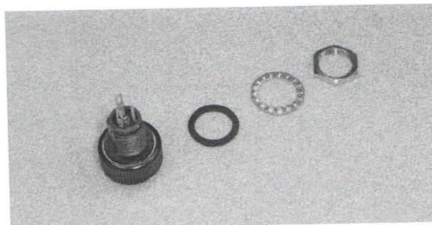
7. Push the control pot through the central hole in the front of the case. Ensure the control pot is correctly orientated (Large tab to the top side of the case).
