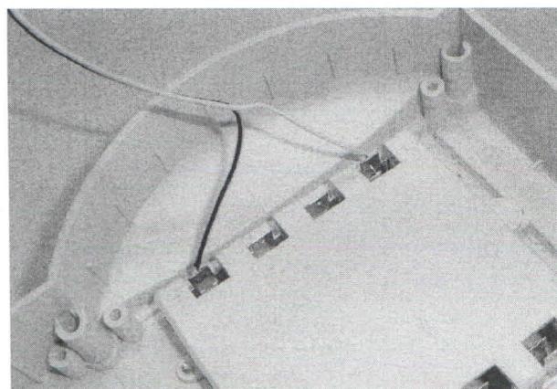
16. Connect the 2 pin M22 connector to the 2 pin connector on the PCB.
