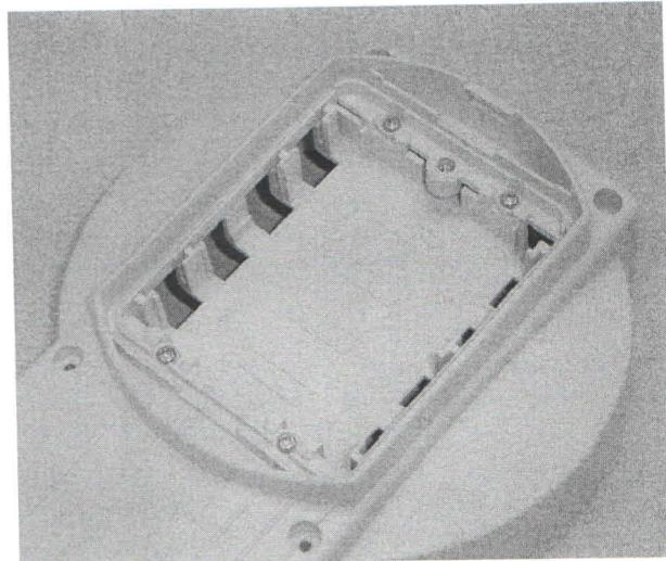
5. Insert the battery contacts from the back of the case.
