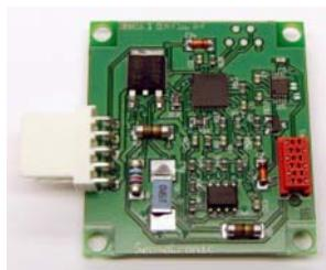
The OEM-Flow A-F module has been designed for measuring the breathing gas flow in respiratory and anaesthesia machines. It works with state-of-the-art hot-wire flow sensors.
