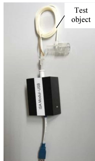
UART-USB-Converter for mainstream CO 2 UART-USB-Converter with integrated IRMA-Sensor as reference side stream CO 2 ISA-module
