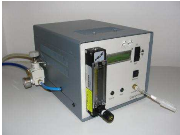
CapnoCheck , CO 2 -Respiratory-Simulator
