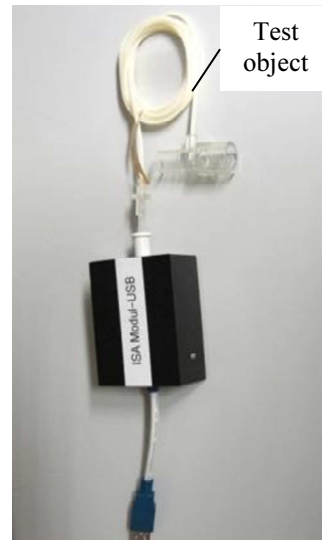
UART-USB-Converter for side stream CO 2 ISA-Sensor
