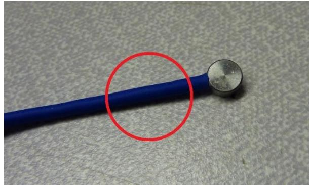
SN: V150110407 – The temperature sensor has been tested. The sensor is open circuit. The sensor head has come away from the cable, but remains attached by the braiding and internal wiring.
