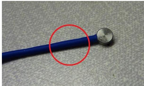
SN: V150110481 – The temperature sensor has been tested. The sensor is open circuit. The cable at the sensor head feels empty. It is likely that the sensor head has come away from the wiring.
