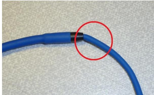
SN: V150110397 – The temperature sensor has been tested. The sensor is open circuit. The cable at the sensor head feels empty. It is likely that the sensor head has come away from the wiring.
