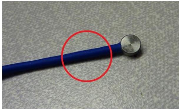
SN: V150110398 – The temperature sensor has been tested. The sensor is open circuit. The cable has an intermittent break at the cable joint.
