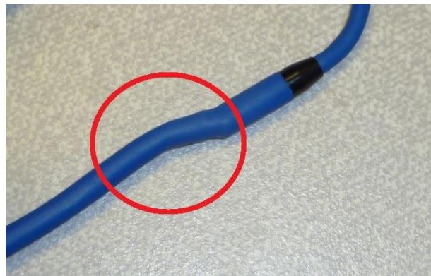
SN: V150110480 – The temperature sensor has been tested. The sensor is open circuit. The cable at the sensor head feels empty. It is likely that the sensor head has come away from the wiring.
