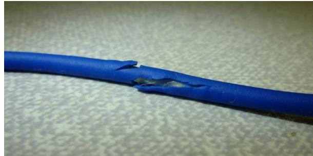
SN: V150110406 – The temperature sensor has been tested. The sensor is open circuit. The cable at the sensor head feels empty. It is likely that the sensor head has come away from the wiring.
