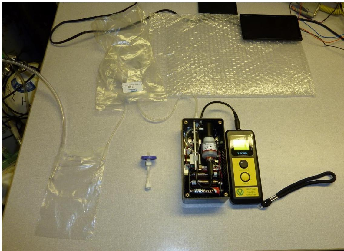
The test would measure the time it took the gas sample to reach the pump box/analyser by observing the Oxygen rise as displayed on the analyser. The test required that the gas to be sampled was not pressurised, so that gas was not pushed down the sample line. The sample time must be from the pumps draw alone. A sample bag, containing Oxygen, was lightly inflated for this purpose and flushed out with air after each test. A five-metre sample
