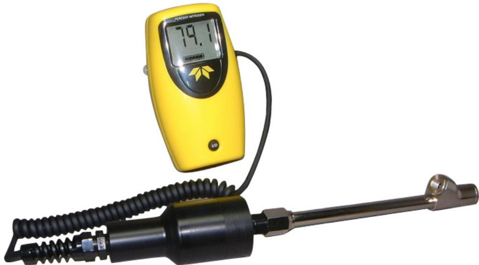
**The AN300 Derived Nitrogen Analyser is a hand-held device designed to analyse the balance of nitrogen in vehicle tyres where nitrogen has been used as an inflation gas.**
