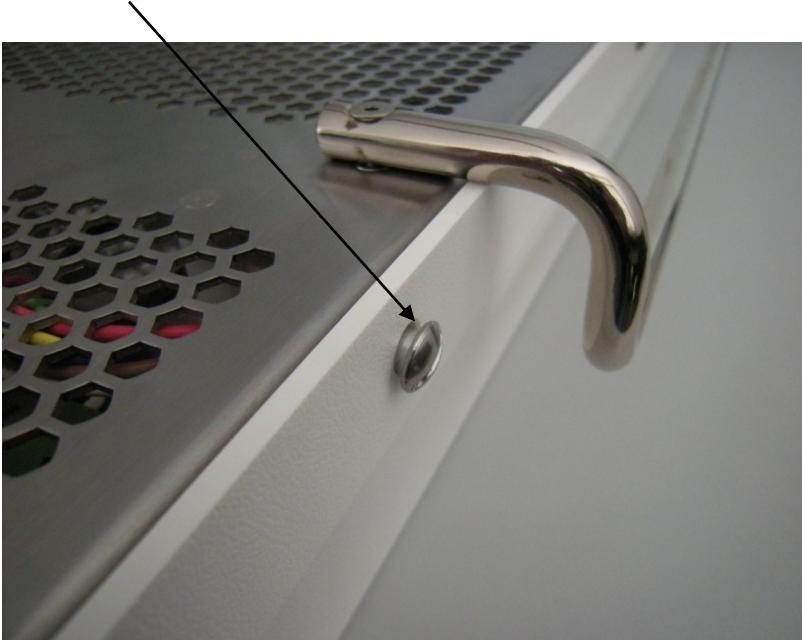
Using a screwdriver, tighten by hand until the screw stops. The screw head should be tightened against the supporting sleeve, not against the casing.
