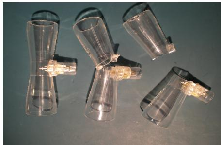
Our risk assessment resulted in determining that there was no risk to the patient, as the flow sensors snapped - either upon removal from service, or possibly during cleaning procedures. The flow sensors are designed as single patient use, so would either be disposed of, or cleaned and tested for further use on the same patient.
