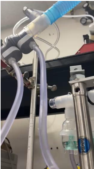
Mounted existing orifice into 3D Printed housings with collection basins and drain fittings
