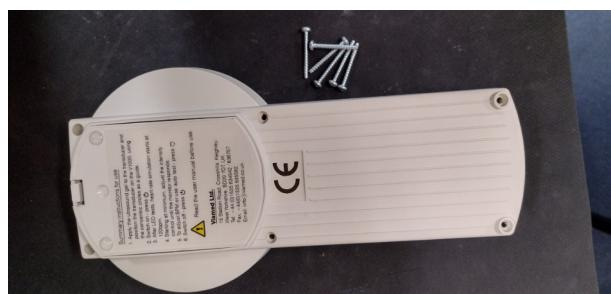
Split the two halves. Take care, the power lead will be connected between the halves.
