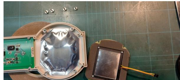
Peel off the old transducer interface cushion. Replace the double sided tape if necessary. Affix a new transducer interface cushion in the space between the support posts.
