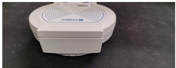
Using the Phillips screwdriver remove the 6sixscrews that hold the two halves together
