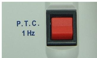
To initiate P.T.C stimulation, press and hold Selector 2 in the P.T.C. 'up' position. The Microstim DB3 will deliver the correct sequence of stimuli; 50 Hz for 5 seconds, a 3 second pause, followed by 1 Hz stimuli. An interval of at least 5-6 minutes should be permitted between successive estimations of P.T.C.
