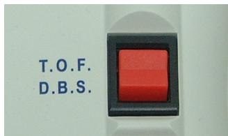
To initiate Train of Four stimulation, press and hold switch one in the T.O.F. 'up' position. The Microstim DB3 delivers the correct sequence of stimuli; four stimuli at a frequency of 2 Hz.
