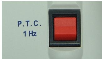
To initiate 1 Hz stimulation, press and hold Selector 2 in the 1 Hz 'down' position. The Microstim DB3 will deliver the correct single stimuli applied repetitively at a frequency of 1 Hz whilst the Selector 2 is maintained in the down position.
