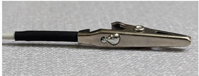
10) Using pliers, fold the retaining tabs over the heat shrink.
