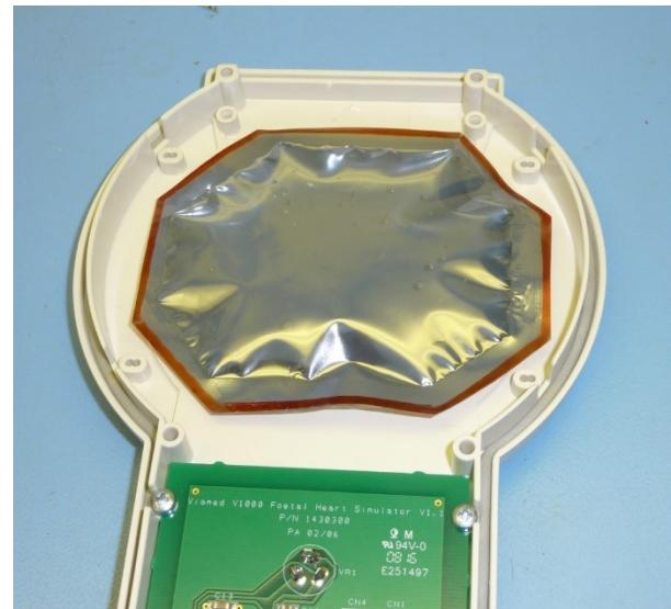
12. Place the transducer assembly over the interface cushion, with spacing nut on the underside of the mounting board, and fix into place using the mounting screws.
