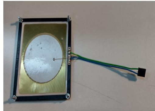
8. Mount the transducer to the transducer mounting board. Space the transducer away from the board using a nut.
