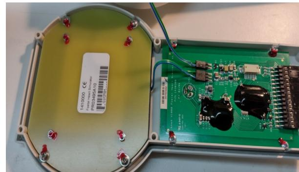
22. Affix a serial number label to the inside of the battery compartment door.
