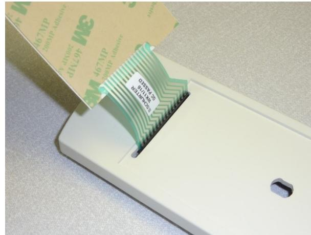
5. Centrally locate the keypad membrane into the recess on the front of the case. Ensure that the bottom edge of the keypad is as close to the bottom edge of the recess as possible.
