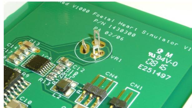
3. Using the PCB retaining screws, affix the PCB into place.
