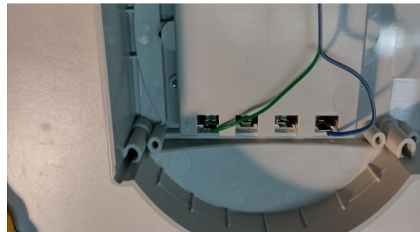
16. Connect the 2 pin M22 connector to the 2 pin connector on the PCB.
