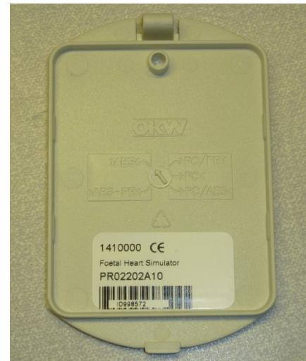
23. Affix a trimmed serial number label to the inside of the battery compartment.
