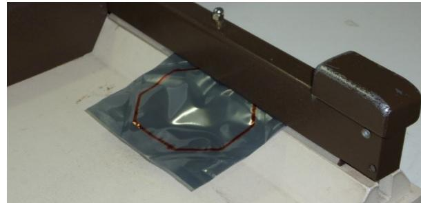
3. Fill the transducer cushion with water, leaving as little air in the cushion as possible, and seal.
