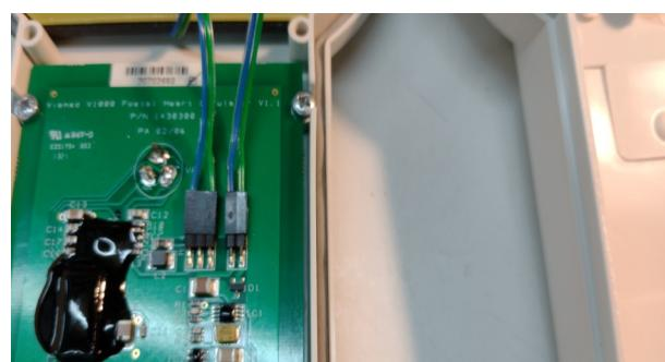
17. At this point, test the unit. Insert 4 x AA batteries and fix the case halves together.
