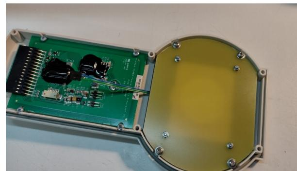
13. Connect the transducer assembly to the PCB using the 3 pin connector.
