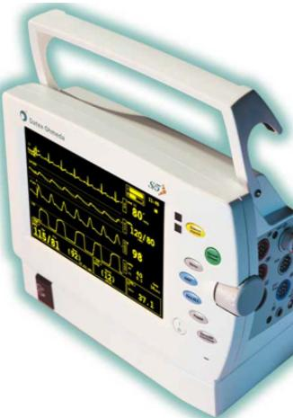
A portable GE Datex-Ohmeda S/5 Light patient monitor. It has a small color display showing ECG, blood pressure, and oxygen saturation data. Below the display is a control panel with several buttons and a small screen.                                                                                                                          | Uses Nicolet connector.<br>Can use Datex style:<br>0014606<br>0014706 |
