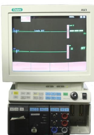
A Datex AS/3 patient monitor. It features a larger color display and a more complex control panel with multiple buttons and knobs. The display shows ECG leads I, II, and III. A text box below the monitor states: "This version AS/3 shown with a module that uses the Nicolet connector, but version may exist that have been upgraded to FM port". | Uses Nicolet connector.<br>Can use Datex style:<br>0014606<br>0014706 |
