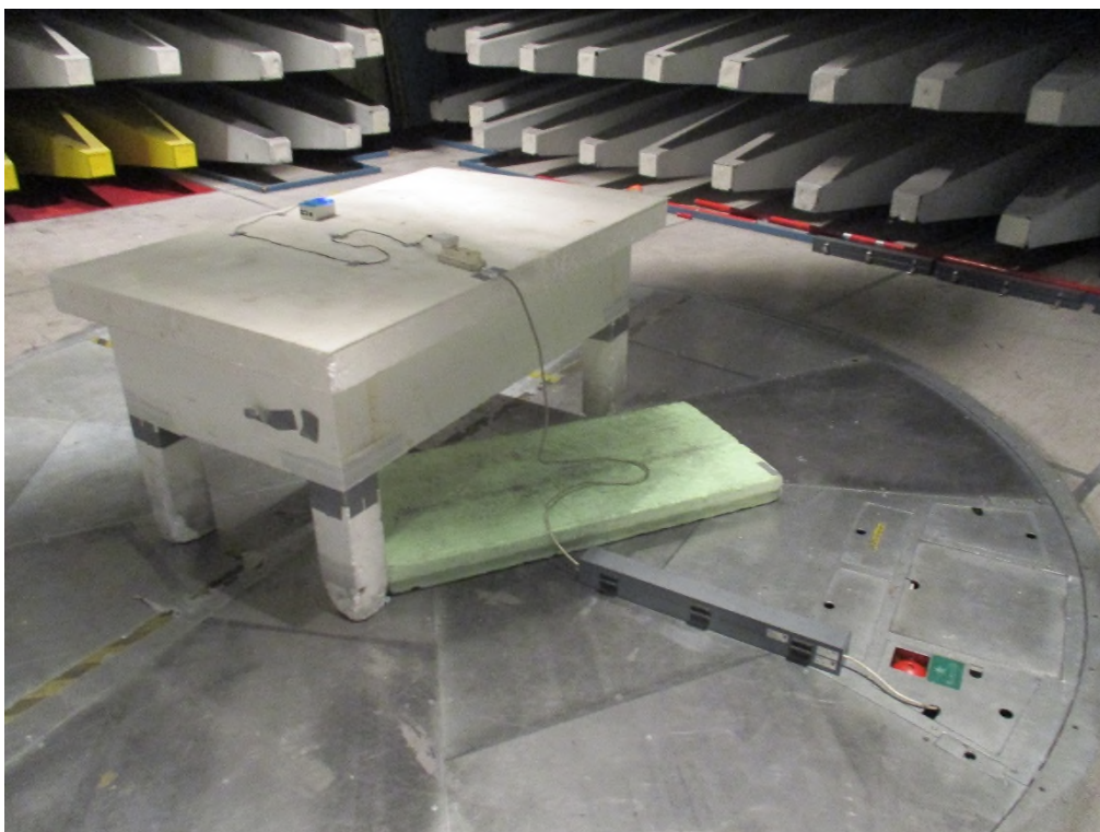
Photo 4.5.2 Test setup regarding measurement of radio frequency electromagnetic field.
