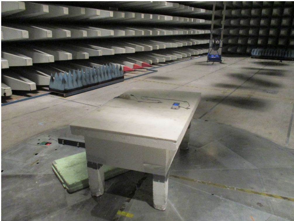
Photo 4.5.1 Test setup regarding measurement of radio frequency electromagnetic field.
