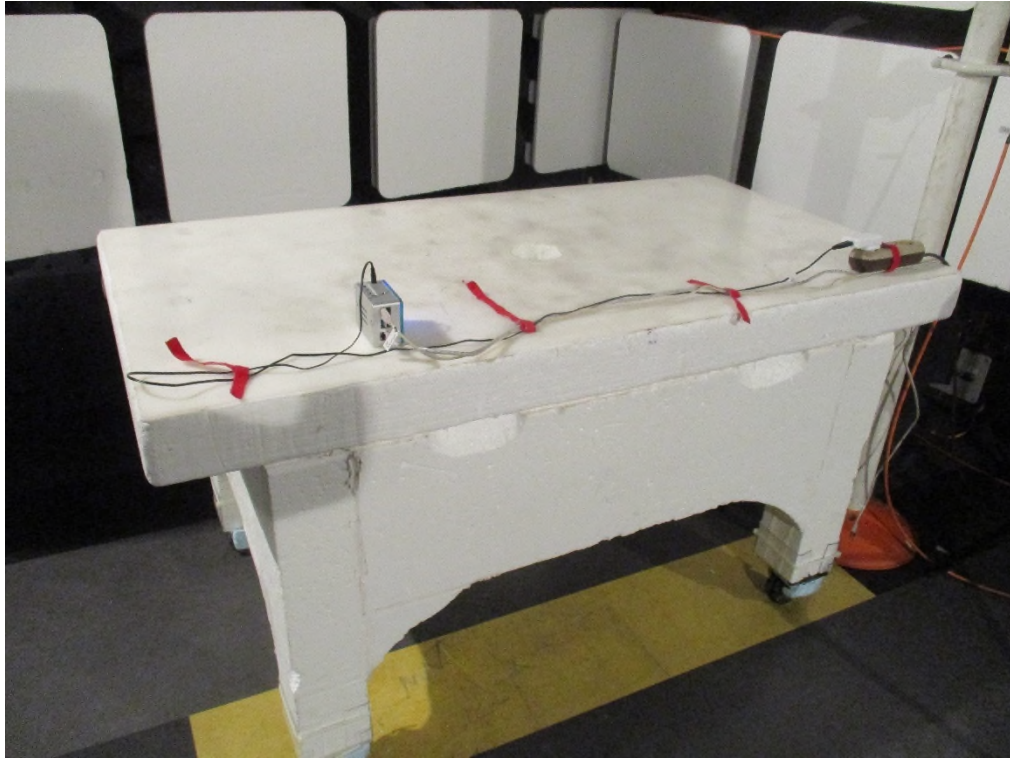
Photo 4.2.3 Test setup regarding immunity to radio frequency electromagnetic field. Side 3.
