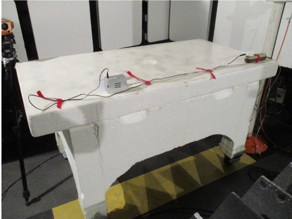
Photo 4.2.5 Test setup regarding immunity to radio frequency electromagnetic field. Side 5.
