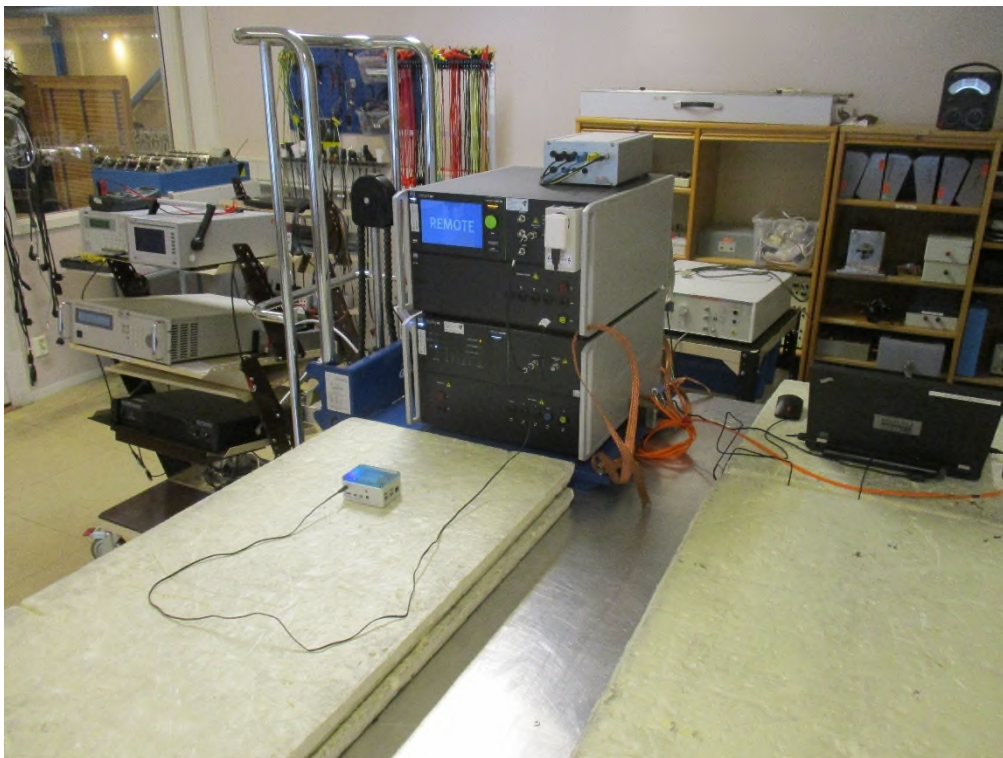
Photo 4.4.1 Test setup regarding immunity to AC mains voltage dips and interruptions.
