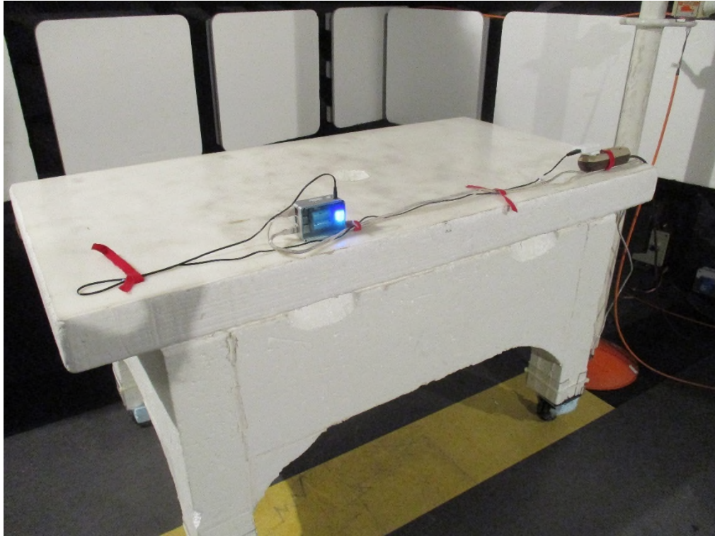
Photo 4.2.1 Test setup regarding immunity to radio frequency electromagnetic field. Side 1.
