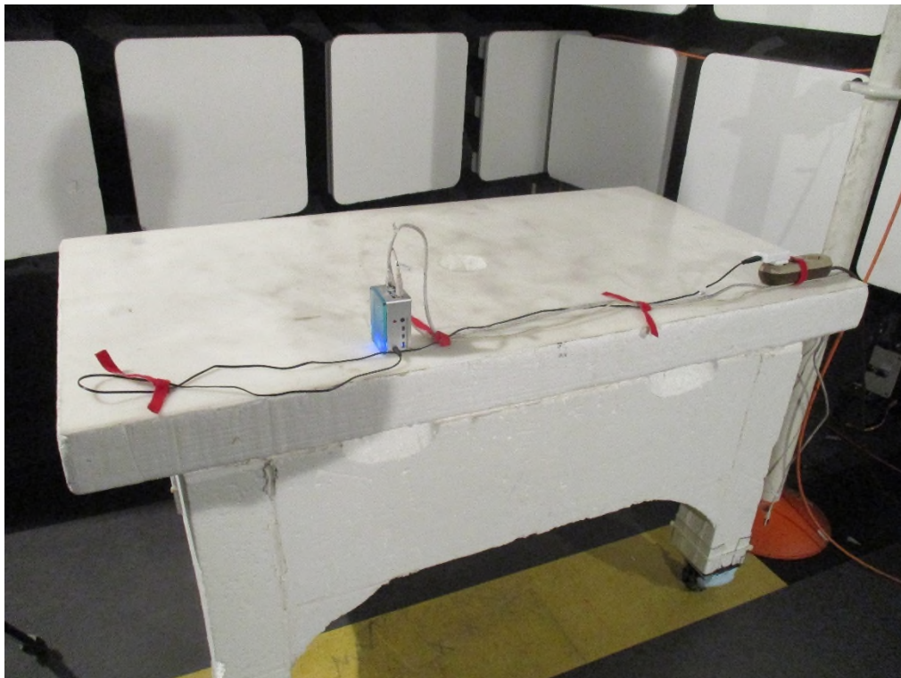
Photo 4.2.4 Test setup regarding immunity to radio frequency electromagnetic field. Side 4.
