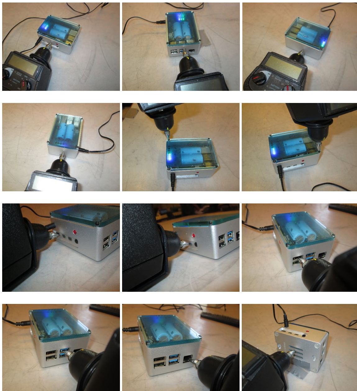
Photo 4.1.2 Test points regarding immunity to electrostatic discharges. Contact discharge test.
