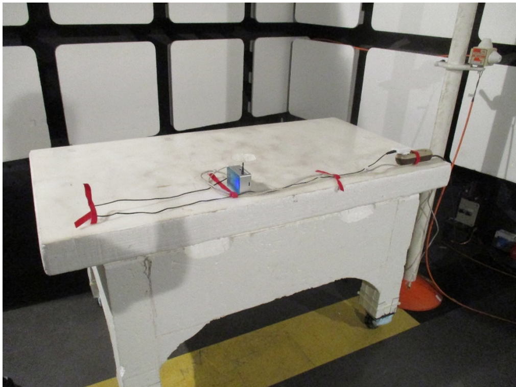
Photo 4.2.2 Test setup regarding immunity to radio frequency electromagnetic field. Side 2
