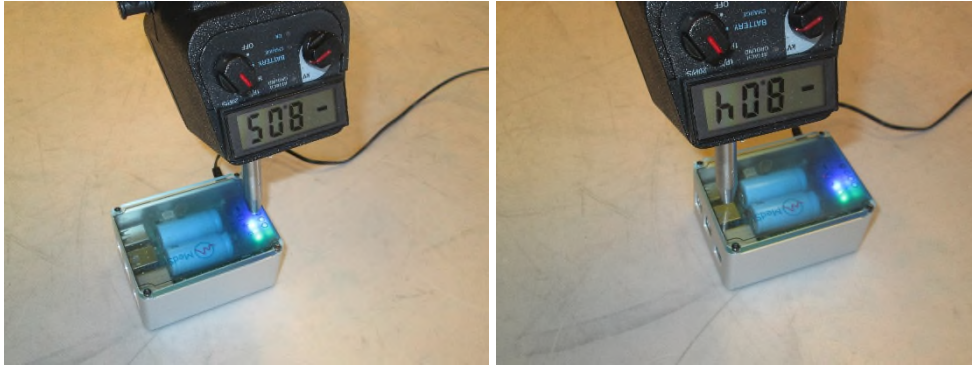
Photo 4.1.4 Test points regarding immunity to electrostatic discharges. Air discharge test.
