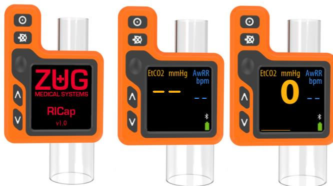
**Figure 6.** Starting up RICap® – Rapid Intervention Capnograph
