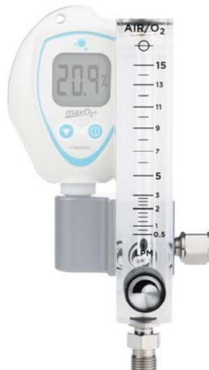
The **BlenderBuddy 2** can be supplied on its own or with a MAXO2+A Oxygen Analyser.
