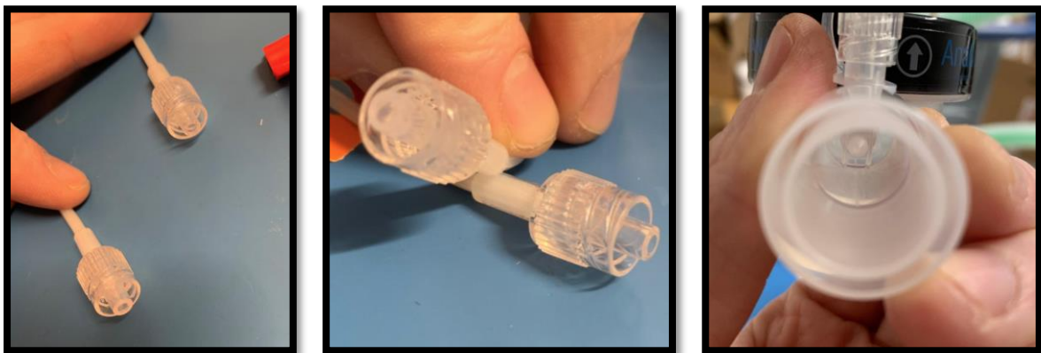
Figure 3 – Images after 72hrs (no material degradation or residue)
