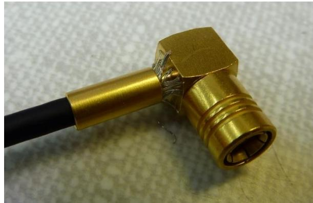
16) Using the pick, tuck any excess shield into the crimp. Push the crimp up to the connector body. The crimp must be flush to the connector body with no strands of shield showing.
