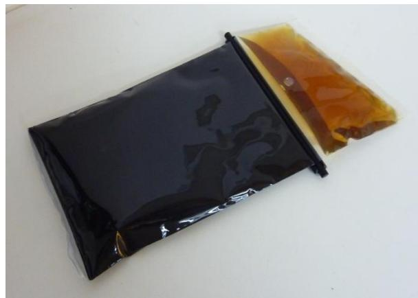
25) Before opening the resin bag, wear rubber gloves and an apron. The resin is very hard to wash off.
