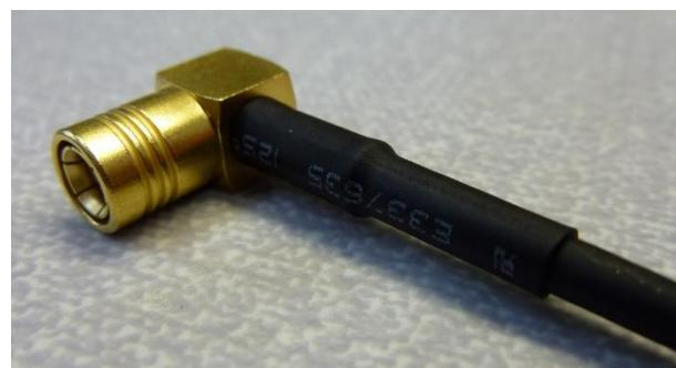
34) Inspect the cables for over spill of resin and general appearance.
