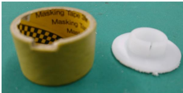
Image2 Spacers for applying pressure
