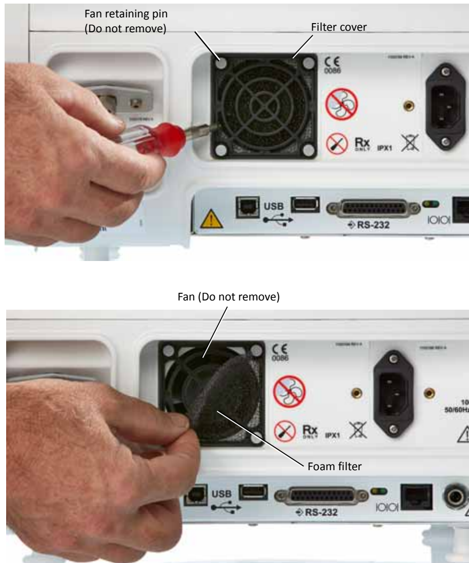
Figure 10-11: Replacing the cooling fan filter
