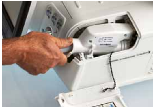
Figure 10-15: Aligning the eSYS cartridge
