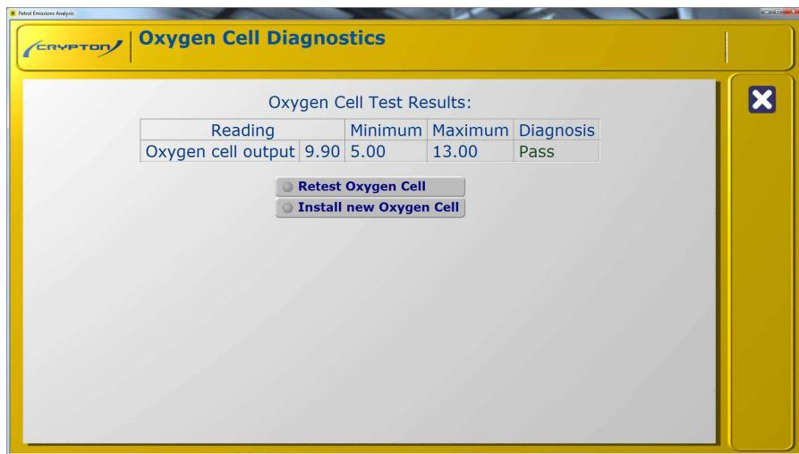
The Oxygen cell output is the voltage measured at the last Autozero. In normal operation the output must fall between 5 and 13 millivolts. For installation of a new cell, the software automatically tightens the limits to between 7 and 13 millivolts.
