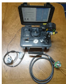
6 Custom cell checker, shown with datalogger interface.JPG 678K
