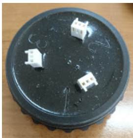
Pot cap with Molex connectors.JPG 1070K
