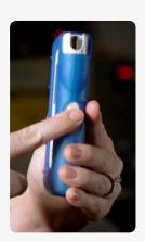
The design also **makes checking outlet pressure extremely simple.** Covering the outlet port with your finger will switch the reading from displaying %O2 & flow rate to displaying the pressure of the O2 concentrator.
