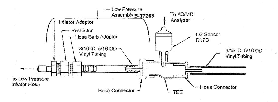
Figure 2-10: Low Pressure Gas Sampling
