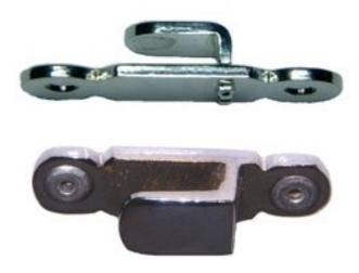
The door component of the catch also suffered from weakening over time: again this was a 2-part construction with the swivelling part affixed to the base plate, by what appeared to be a process of hammering the pin flat once through the base.
