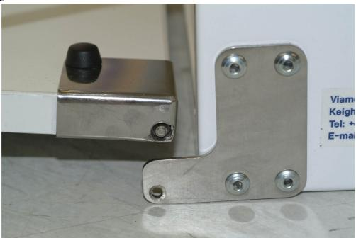
The hole needs to be drilled to a precise depth, or an alternative solution needs to be implemented. Additionally, the weld connecting the pin to the L-bracket needs to be sufficiently robust so as to not allow failure in this manner when subject to excessive loads and/or lateral movement.
