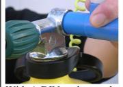
With A DIN outlet gently push the dome into the DIN thread
