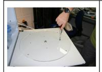
Lift the base unit and clean away any debris left from the drilling. Then replace the base unit onto the platform and insert the screws through the holes in the base unit into the pre-drilled holes in the platform and tighten.
