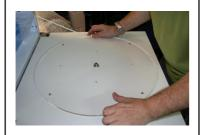
Place the base section of the rotating bed with the central hub in place, onto the platform. Looking through the base section, line up the furthest tip of the central hub with the horizontal line and the line up 2 x of the screw holes with the vertical line.
