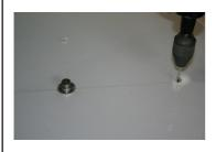
Through the 4 screw holes, making sure that the base does not move, drill small pilot holes into the platform.
