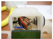
We need to cut away the body to accommodate the side edges of the two flat connectors. PCB on its way to you today
