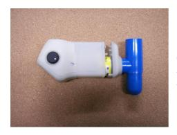
The enclosure needs to be lengthened by another 10mm to allow big hands to hold it. The spare volume inside will be above the jack connector and can be used in subsequent designs.
