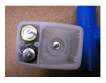
The collar needs to be removed so that the Jack plug can be locked otherwise it will rotate with the sensor
