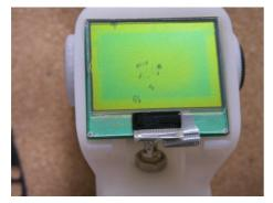
The recess for the LCD and PCB needs to be larger. i.e 38.3 mm x 33.3mm
