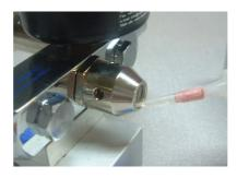
11.<u>TT pressure gauge accuracy check</u>: Cover the T piece adapter port and increase the flow of gas to achieve a displayed reading of 30 cm $H_2O$  on the TT pressure gauge. Ensure a reading of  $\pm$  2% of the Precision Valve Reading on the digital manometer and record
