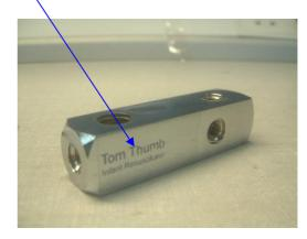
a). Insert diamond copper washer into the single threaded hole on the label side of body block.
