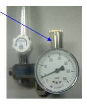
8. Place a thin O ring over the threaded end of the 15mm outlet. Screw the 15mm outlet into the threaded hole in the right face of the body block. Use the adjustable spanner to tighten.
