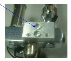
12. Attach rail clamp to the spacer block using 2x M4x10mm hex drive bolts.
