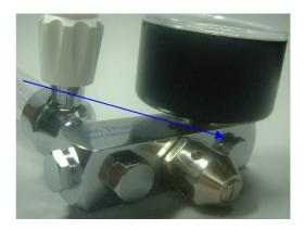
7. Place a thin O ring over the threaded end of the adjustable valve. Screw the adjustable valve into the remaining threaded hole in the top face of the body block. Use the adjustable spanner to tighten.
