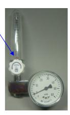
5. Line the thread of the precision valve with two complete layers of PTFE tape, place a thin O ring over the thread, and screw into the centre bottom threaded hole. Use adjustable spanner to tighten.
