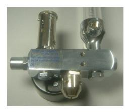
10. Line the thread of the inlet hose right angle adapter with two complete layers of PTFE tape and screw into the rear of the flowmeter ensuring that the right angle adapter is vertical, tight and cannot be moved by hand.
