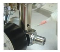
9. Check for TT pressure gauge sticking: Release and cover the T piece adapter port a number of times, ensuring that TT pressure gauge returns to 23 - 27 cm $H_2O$ . Uncover the precision valve holes.
