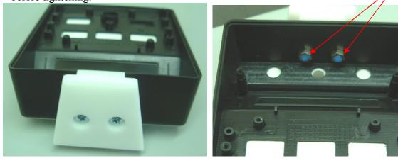
14. Fasten reset button to the upper case (take care not to over tighten).
