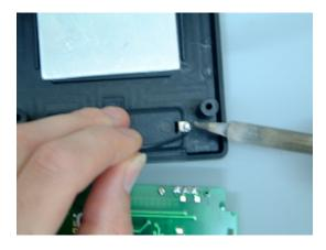
4. Cut all three wires at the topside of the green circuit board flush.
