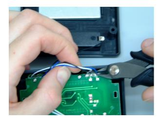
5. Remove circuit boards from the upper casing, and protective film from the display face.
