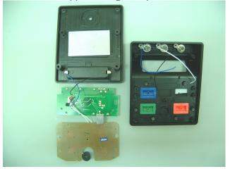
6. Remove three M5 nuts from the upper casing. Keep any one wire for use further in the assembly process.
