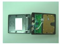
2. Disassemble circuit board and position bar via fastening screws.
