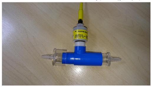
This system would allow you to add your tubing to either side of the TEE, having the barbed connector on the other side eliminates a potential venturi effect which could lead to a diluted reading, but will still allow the gas to escape and not create too much back pressure.
