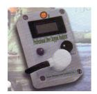
Based on Analox. This analyser uses the Analox style 9212- sensor. The sensor is distinctive in having a "Pipe" fitting in place of the normal screw thread and uses a push fit to connect the sampling tube. The sensor output is typically 25mV.
