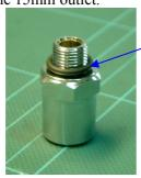
1. Unscrew the hose from the right angle adapter and the right angle adapter from the flowmeter. Remove the original PTFE tape from the right angle adapter, rewind with 2 complete layers of new PTFE tape and refit the adapter vertically into the flowmeter.
