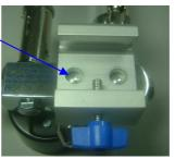
9. Remove the original PTFE from the inlet hose threads and right angle adapter. Line the thread of the inlet hose with two complete layers of new PTFE tape and refit the hose into the inlet hose right angle adapter using 12mm open-ended spanner ensuring it is tight.
