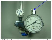
3. Unscrew the blanking bolts from the threaded left side hole and remaining threaded hole on the bottom face of the body block respectively. Ensure the ports, and threads, are free of foreign matter. Replace the thin O-rings (p/n 0330214) on the blanking bolts and refit into the body block.
