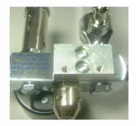
2. Detach the spacer block from the body block.
