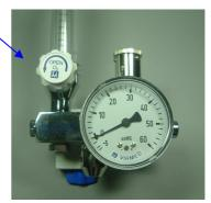
6. a). Unscrew the pressure gauge. b). Ensure the port and threads are free of foreign matter. c). Insert a new diamond copper washer into the single threaded hole on the label side of body block. d). Screw in the pressure gauge and use the 14mm open ended spanner to tighten; the gauge should appear straight in comparison to the block and not able to be removed without the aid of tools.
