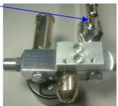
2. Unscrew the adjustable valve from the right hand threaded hole on the top face of the body block. Ensure the port, and threads, are free of foreign matter. Disassemble the adjustable valve and re-grease the valve seat and valve screw. Replace the thin O-ring (p/n 0330214) and refit the valve.
