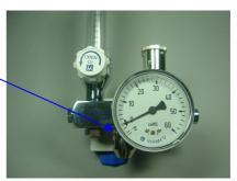
5. Unscrew the Flowmeter and remove the flowmeter bolt from the right hand non-threaded hole in the body block. Ensure the port, and threads, are free of foreign matter. Replace the thin O-ring (p/n 0330214) & thick O-ring (p/n 0330213) and refit the flowmeter bolt and flowmeter.
