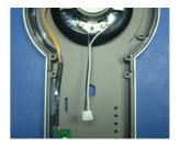
39. Starting at the bottom, apply the overlay panel ensuring that no air pockets are formed. Apply pressure gradually working toward the top, feeding the flexible cables through the slots in the case as appropriate.
