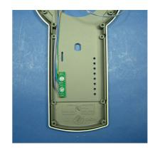
29. Grind away the 2 mounting points in the upper case half as shown.
