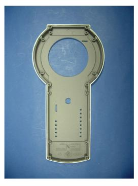
21. Black out the area immediately around the left hand row of 8 x 3mm holes with permanent marker. Stick double sided tape to cover the majority of recessed area of the upper case half. Trim tape to suit.
