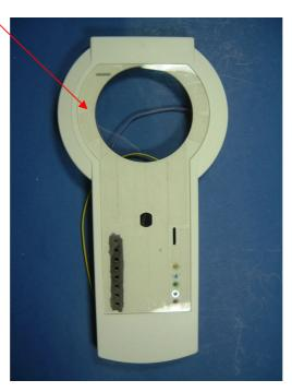
32. Using appropriate drills and files, duplicate the hole in the enclosure for the intensity pot and the two slots for the flexible connectors in the overlay back panel. Drill a hole in the centre of the transducer area to allow the nozzle of the syringe to be passed when filling the transducer with silicon fluid. Ensure that all swarf is removed (use tooth brush or such like) and the upper side of the top panel is ground perfectly flat where slots and holes fall (no sharp edges etc.).
