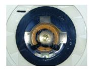
38. Solder a 2 way ribbon cable (white / black) to the speaker terminals; white-positive, black-negative. Fit a 2.5 molex connector to the cable ensuring the overall length of 70mm cable assembly.
