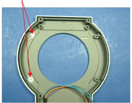
30. Sleeve 50mm of wiring harness with black heat shrink tube. Allow the yellow/orange combination to exit the wiring harness, and sleeve a further 40mm of wiring harness (leave an 8mm gap between lengths of heat-shrink). Allow the purple/grey combination to exit the wiring harness and heat-shrink a further 50mm of the blue/green combination. Glue the wiring harness to the upper case half at the points shown with hot glue.
