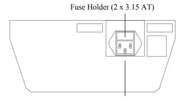
Input Socket for Mains Cable (220-240V AC, 50Hz)
