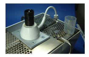
8. Connect & lock the Wandarm to the radiant warmer  $\Rightarrow$  Wandarm adapter and extend the arm.
