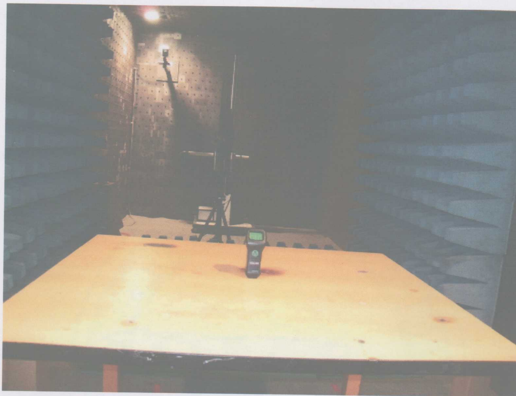
Photo 4 Radio Frequency Electromagnetic Field Immunity Test
