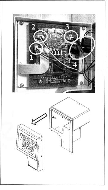
4 Gently peel up the alarm from the case. Carefully clean off any excess adhesive remaining on the surface.
