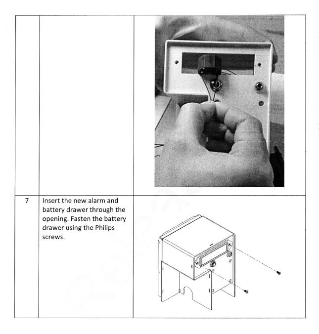
8 Remove the adhesive backing from the new alarm and firmly press down into place over the alarm holes.
