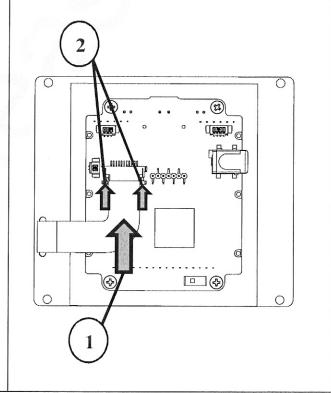
Install the keypad back into the bezel and tighten the selftapping screws down uniformly to ensure proper sealing of the gasket. Note: Use caution not to strip the threads in the bezel. Reattach the front Bezel assembly according to Front Bezel Assembly Installation.
