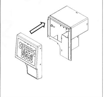
Carefully slide flowmeter 10 blender core assembly into monitor enclosure. Using 5/32" Allen wrench, 11 install the two socket cap screws and washers to the rear of the device and firmly tighten. It is helpful to manually start both screws before fully tightening.
