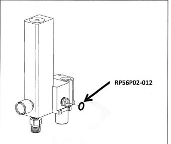
Using a 5/16" Allen wrench, tighten (clockwise) the manifold bolt to the left side blender port to 100 in-lbs.
