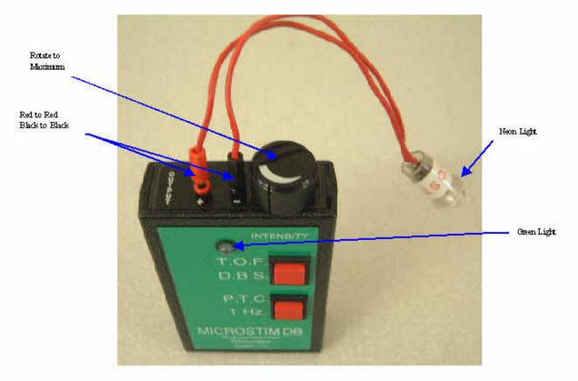
6. Disconnect the Neon Test lead from the Microstim, remove the battery and refit the battery cover. Ensure the unit is serial numbered, the CE label is attached to the bottom R.H. corner of the Instructions for use label and the stock sheets are completed. When packing the unit for despatch, ensure that the box contains the Battery, the Leads and the Operators Manual.
