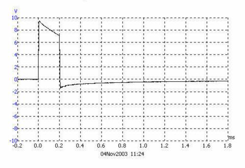
6. Set the intensity control to maximum. Push, and hold, the upper toggle switch to D.B.S. Then ensure that the Microstim gives 3 pulses of 0.2ms width at 20ms intervals (50 Hz), followed by a gap of 750ms, then again, 3 pulses of 0.2ms at 20ms intervals (50 Hz). Then ensure that the intensity control varies the pulse height from approximately 8-10V (peak, leading edge) to 0V. Then release the toggle switch.
