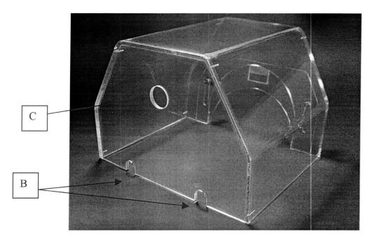
Use the access cutouts in the base (B) to run IV lines or oxygen sensor cables into the Head Box. The 22mm input hole (C) can be used to supply Oxygen via a standard oxygen tube 5mm or a humidified gas using 22mm or 15mm standard fittings
