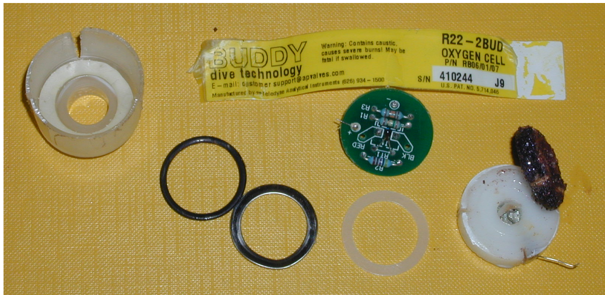
Fig 8-4: Unused R22-2BUD Disassembled, showing electrodes, membrane, housing, and electrolyte suffering from dehydration after storage in a air conditioned laboratory environment. Note the cathode is almost completely black: this is caused by organic contamination in the electrolyte.
