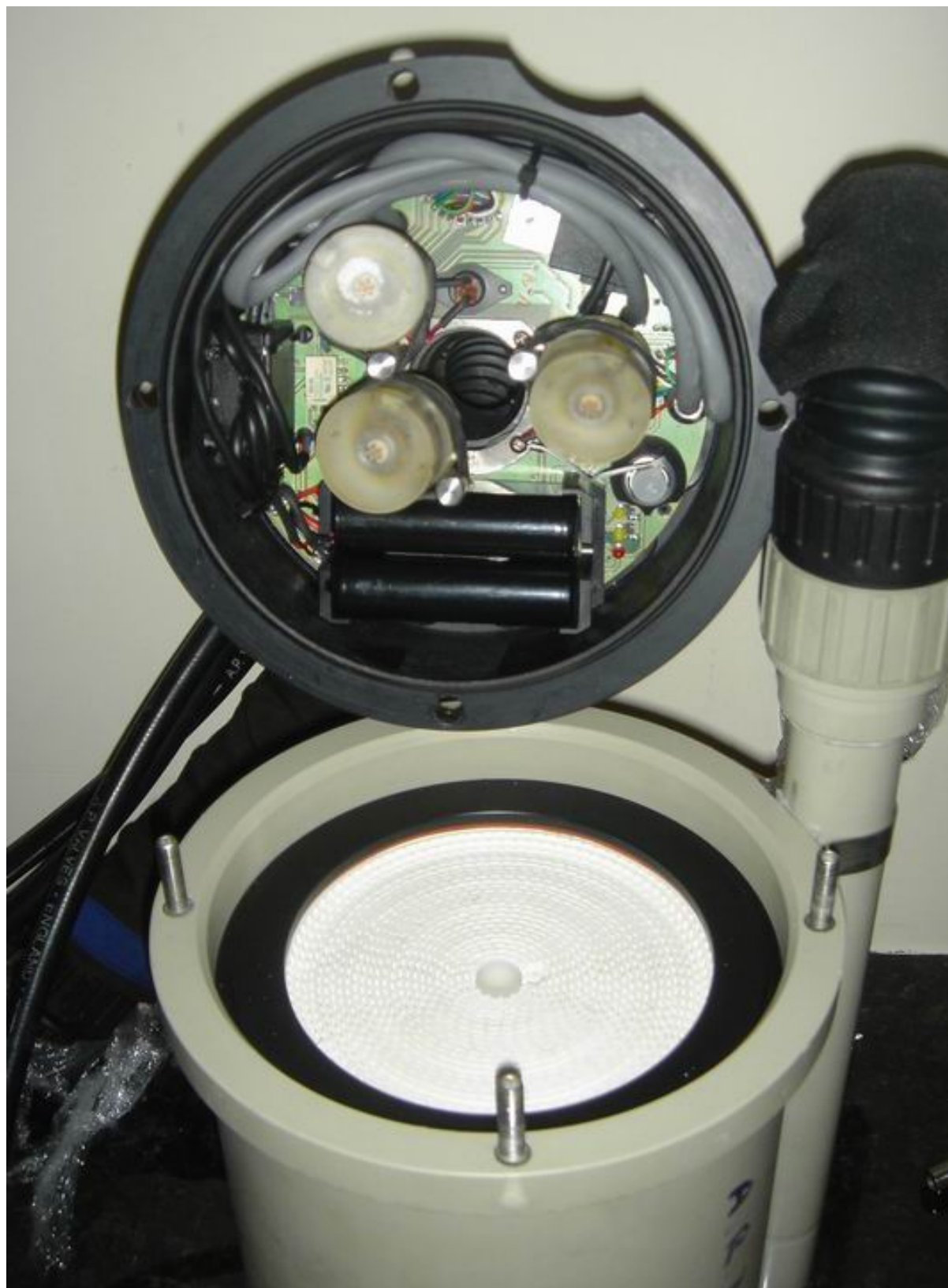
Fig 9-29: Test Rig using an improved AP Valves Inspiration Classic to test the Insovt DK.32s on dives. An ExtendAir scrubber was fitted, the batteries replaced by rechargeable lithium ion cells and the failure point at the top of the lid have been removed by Deep Life.
