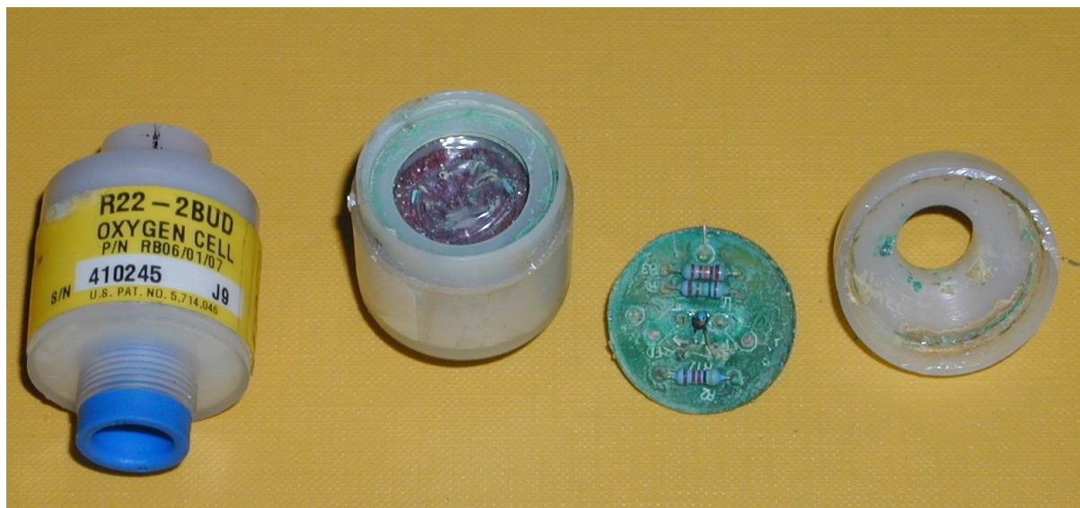
Fig 8-3: Rear side of circuit board after use (S/N 410243), alongside control sensor (S/N 410245). The deposition of KOH can be seen on the membrane as a whitish film.
