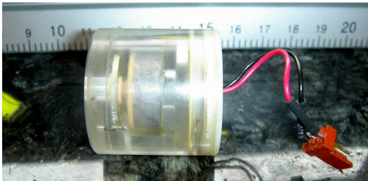
Fig 9-28: Insovt DK-32 with rule and angle showing the thick hydrophobic membrane in front of the cell
