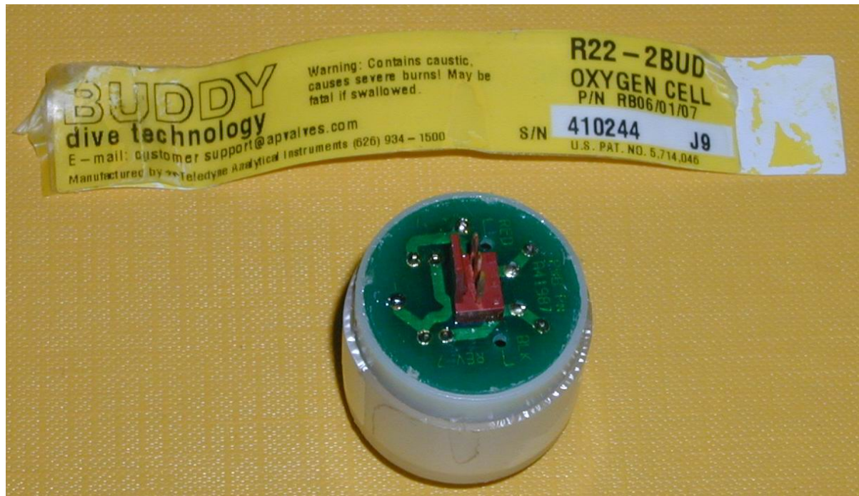
Fig 8-2: R22-2BUD sensor from stored batch, showing circuit board in original condition.
