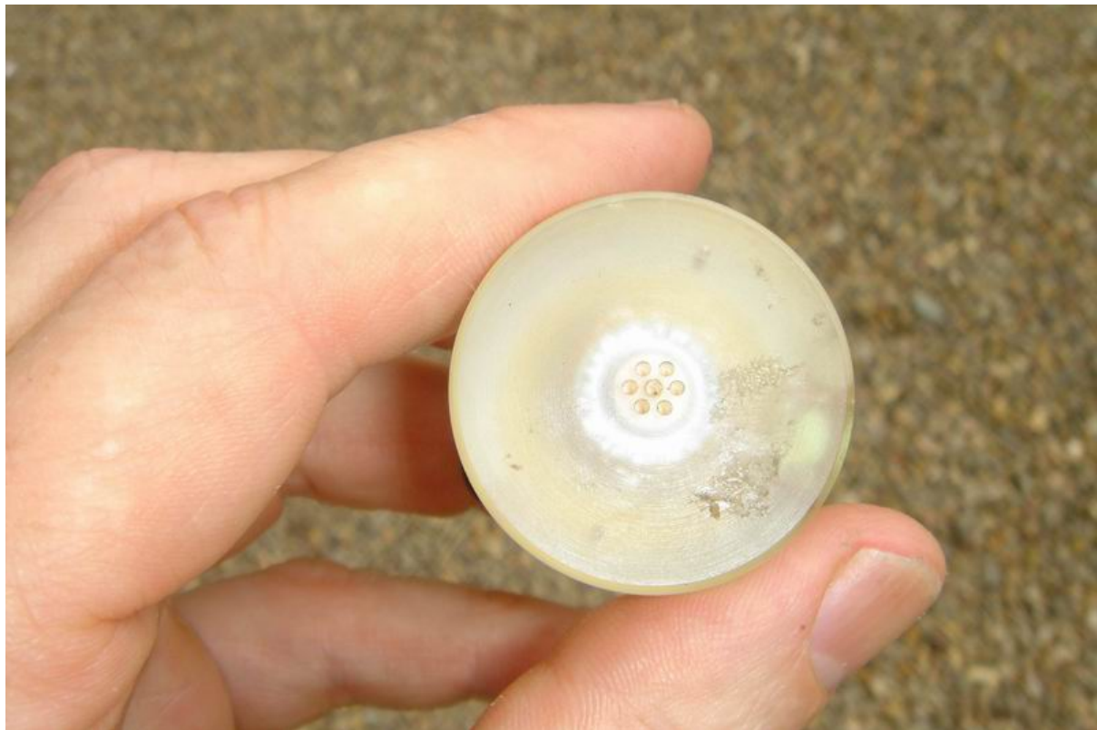
Fig 9-25: Front face of Insovt DK-32 showing integral and thick shield in front of hydrophobic membrane to prevent membrane lifting when depressurised rapidly. Sensor serial number 171, shown after testing.
