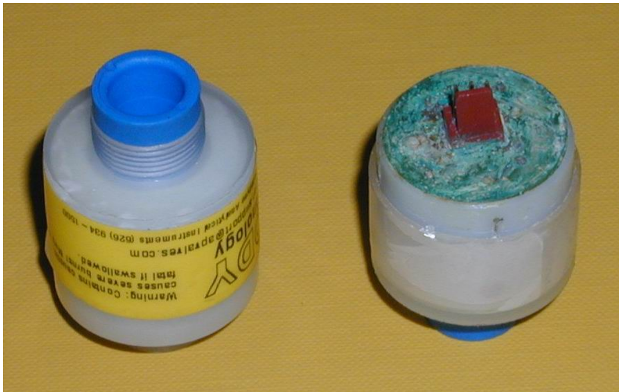
Fig 8-1: R22-2BUD Sensor with rear plastic removed, showing considerable corrosion after 10 hours. This is due to microscopic tears in the rear membrane of the sensor allowing Potassium Hydroxide to be deposited on the pcb and its components.
