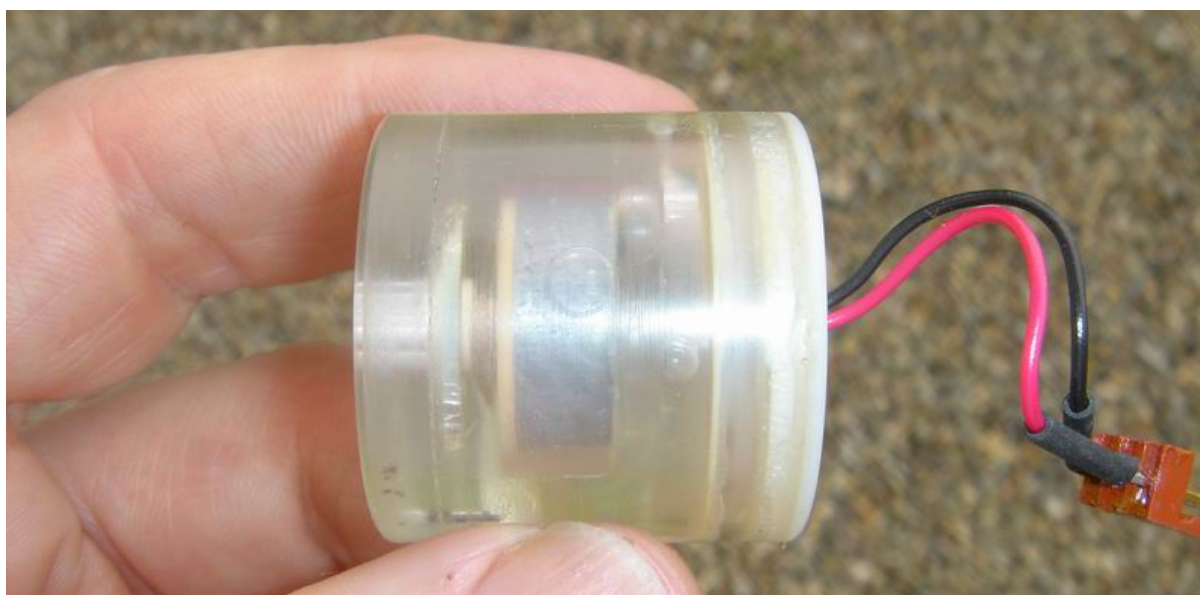
Fig 9-27: Insovt DK-32 showing KOH solution fill: bubble can be seen behind anode and also in second compartment. This shows the two part potting process to avoid contaminants affecting the cell. Note the thick material in front of the cell to prevent depressurisation forcing electrolyte out of the cell.
