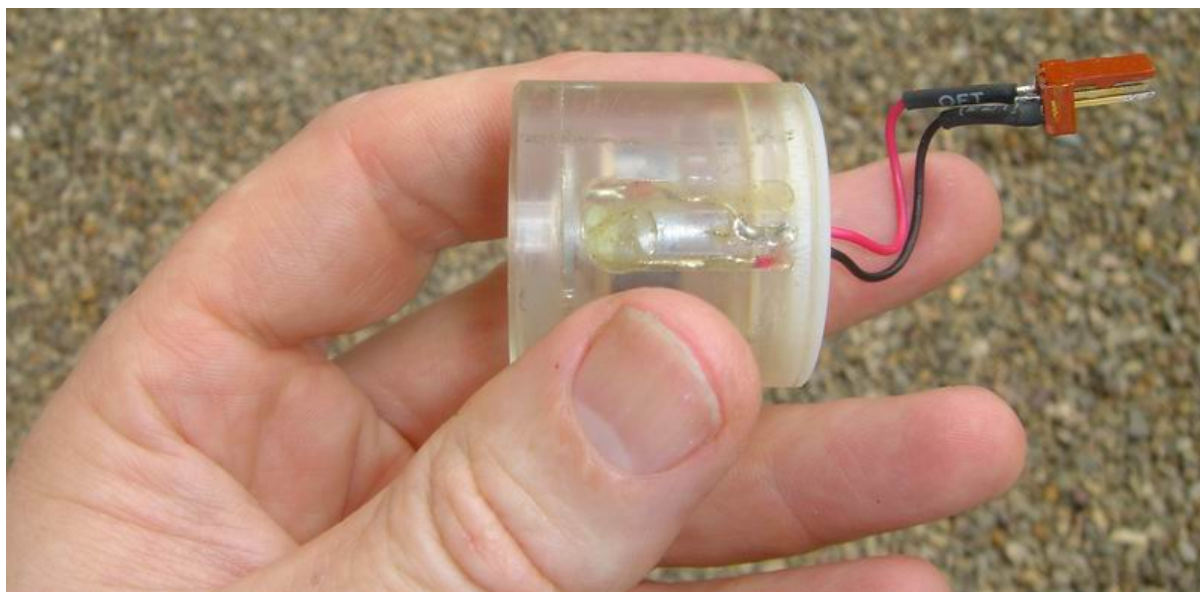
Fig 9-26: Side view of Insovt DK-32 after testing, showing the hard wired temperature compensation circuit potted into housing. Unfortunately it was functioning in reverse, causing a 2%/C change due to a circuit error.
