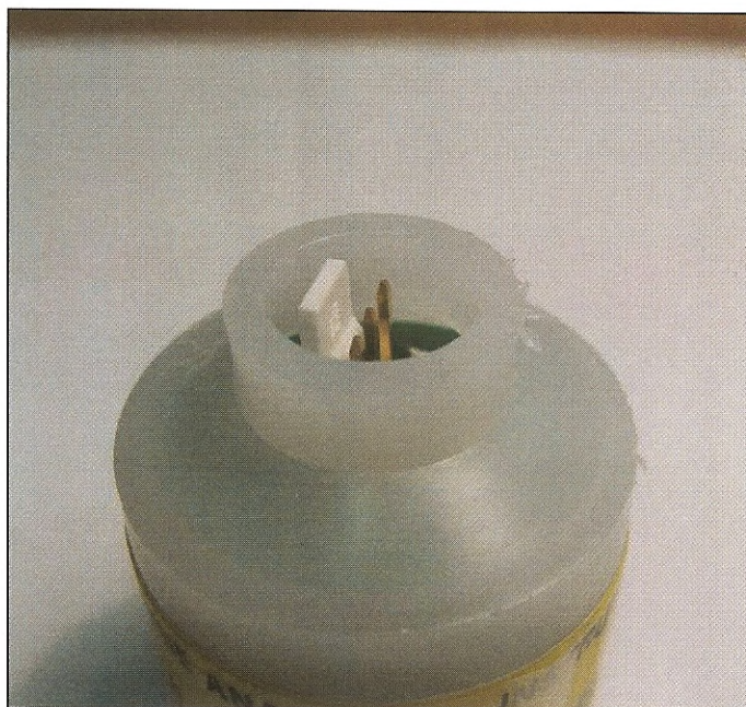
Fig 3-4: There is a small dent near the connector hole of the sensor
