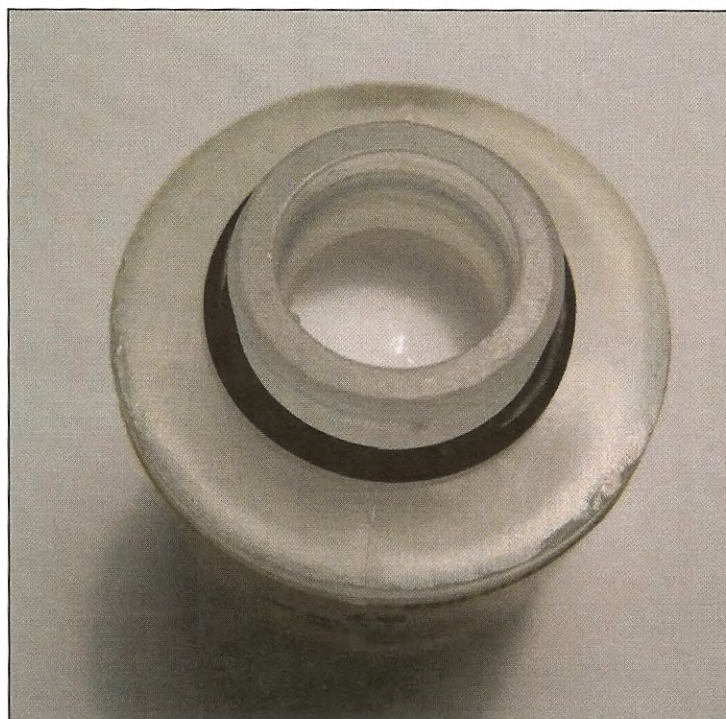
Fig 3-3: Electrolyte drops on the sensor membrane
