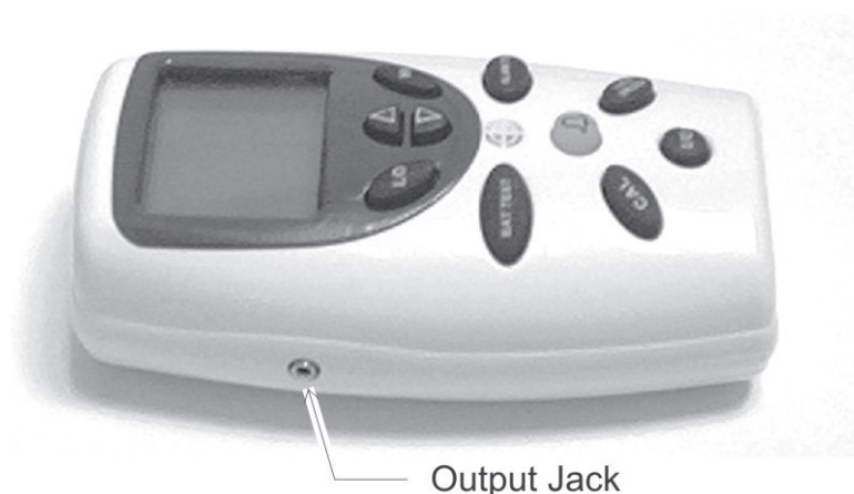
Figure 2-9: 0-1 VDC or RS 232 Digital Output Port
